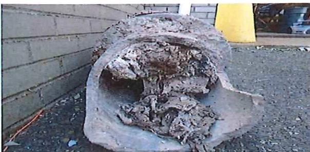
This an 8 inch sanitary sewer main blocked solid by grease, wipes and rags. The replacement of this section of sewer cost \$9,500.00.
